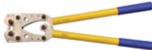
Crimping tool with hexagon dies for tubular copper cable lugs Cable area interval: 16 - 95 mm 2 Part No.: V 0330
