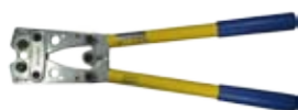
Crimping tool with hexagon dies for tubular copper cable lugs Cable area interval: 6 - 50 mm 2 Part No.: V 0320
